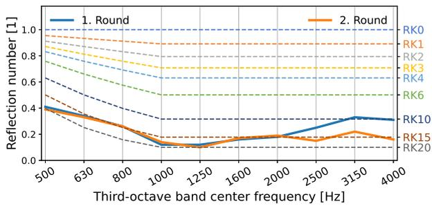
**Figure 4:** Third-octave band-dependent reflection coefficients of a prototype according to DIN EN 1793-5 before and after optimization.
